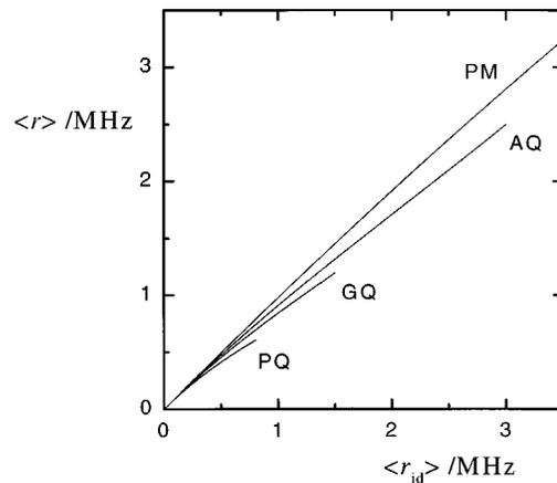
FIG. 9. Transfer functions for Gaussian inputs of the four detection systems, as indicated.
