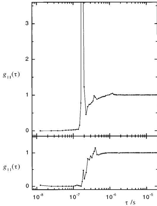
FIG. 4. Photocount autocorrelation functions displaying the direct effect due to detector nonlinearities for the passive quenched APD circuit (PQ). (a) (top): PQ module utilized in this contribution; (b) (bottom): equivalent module with the same specifications as the previous one. The count rates were  $\langle r \rangle \approx 100$  kHz in both cases.
