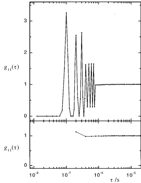
FIG. 5. Photocount autocorrelation functions displaying the direct effect due to detector nonlinearities for the gated quenched APD circuit (GQ). (a) (top): measurement employing the fast board; (b) (bottom): measurement with the conventional correlator board. The count rates were  $\langle r \rangle \approx 100$  kHz in both cases.
