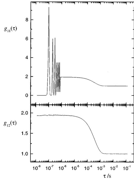
FIG. 7. Photocount correlation functions of the light scattered by a polystyrene latex sample under an angle of 90°, measured with a gated quenched APD. (a) Autocorrelation function, the count rate was  $\langle r \rangle = 89$  kHz. (b) Cross-correlation function, the count rates were  $\langle r \rangle_{GQ} = 170$  kHz and  $\langle r \rangle_{PM} = 170$  kHz.
