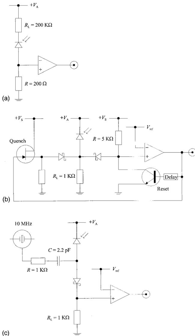
FIG. 1. Scheme of three different electronic quenching circuits. (a) Passive quenching, (b) active quenching, (c) gated quenching.
