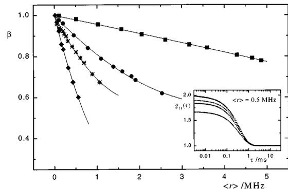
FIG. 8. Intercept  $\beta$  of  $g_{11}(\tau)$  of the light scattered by a polystyrene latex sample under an angle of 90° as a function of the count rate  $\langle r \rangle$ , measured with four different detection systems. The inset shows the respective autocorrelation functions for  $\langle r \rangle \approx 0.5$  MHz. The detection systems shown are from top to bottom: PM (squares), AQ (circles), GQ (stars), PQ (diamonds). The drawn lines are the fitted functions according to Eq. (7).
