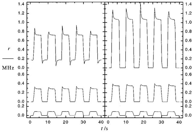
FIG. 2. Measured count rate of the GQ circuit as a function of time, illuminated by a LED chopped with a frequency  $\nu=0.12$  Hz. (a) (to the left): Parameter is the applied voltage  $U_A$ ; from bottom to top:  $U_A = \{222, 224, 226\}$  V. (b) (to the right): Parameter is an increase of the incident light power  $J$ , applying  $U_A = 222$  V; the steady-state count rate  $\langle r \rangle$  is, from bottom to top:  $\langle r \rangle = \{0.09, 0.35, 1.1\}$  MHz.
