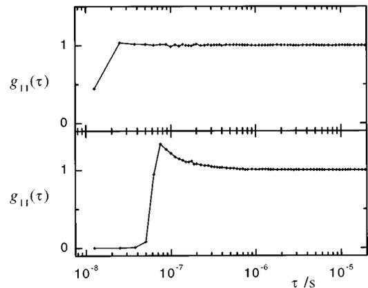
FIG. 3. Photocount autocorrelation functions displaying the direct effect due to detector nonlinearities. The count rates were  $\langle r \rangle \approx 100$  kHz in both cases. (a) (top): Photomultiplier plus amplifier/discriminator (PM), (b) (bottom): active quenched APD circuit (AQ).
