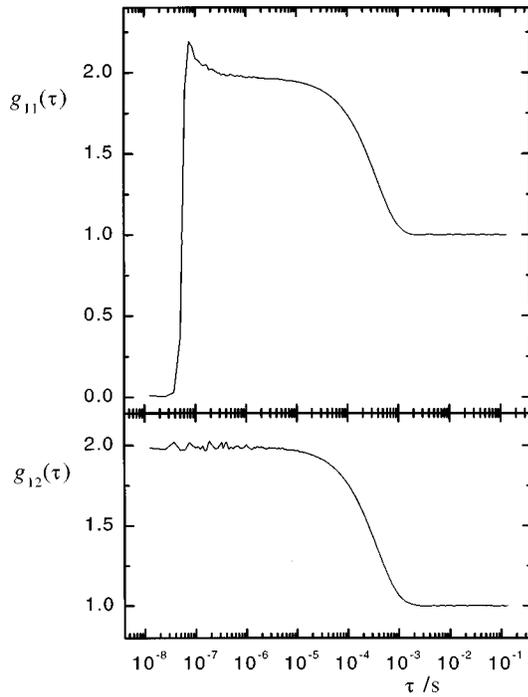
FIG. 6. Photocount correlation functions of the light scattered by a polystyrene latex sample under an angle of 90°, measured with an active quenched APD. (a) Autocorrelation function, the count rate was  $\langle r \rangle = 179$  kHz. (b) Cross-correlation function; the count rates were  $\langle r \rangle_{AQ} = 182$  kHz and  $\langle r \rangle_{PM} = 14$  kHz.
