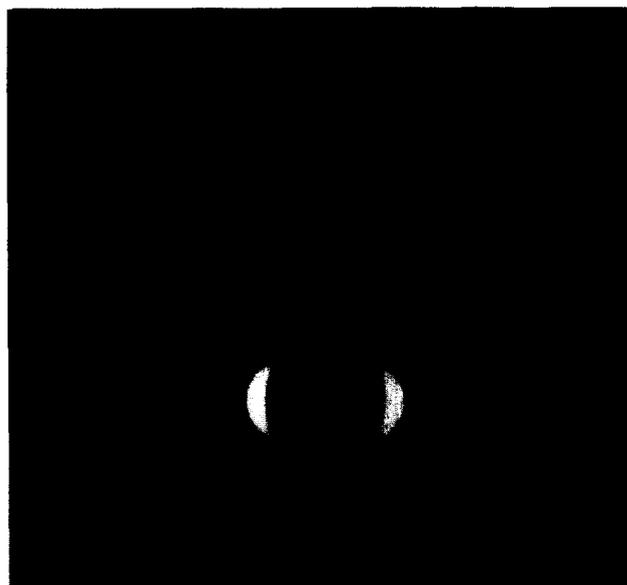
Figure 4 WAXS pattern of a sample stretched at  $T = 100^\circ\text{C}$  with  $\alpha = 4.5$ . The draw axis is vertical
