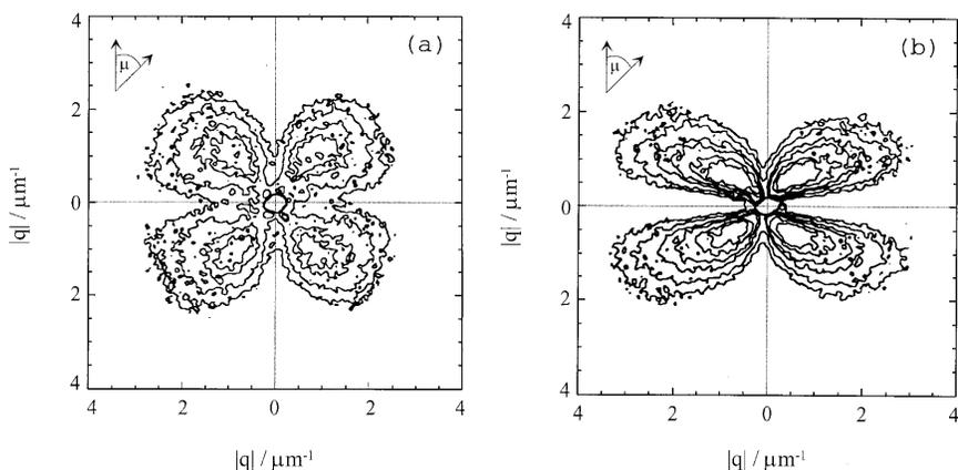
Fig. 6. Depolarized small-angle light-scattering patterns of drawn samples for two different deformation ratios as a function of  $q$ ; the incident light was perpendicular to the fiber axis. (a)  $\lambda_S = 1.4$ ,  $\lambda_M = 1.0$ ; (b)  $\lambda_S = 3.1$ ,  $\lambda_M = 1.8$ .
