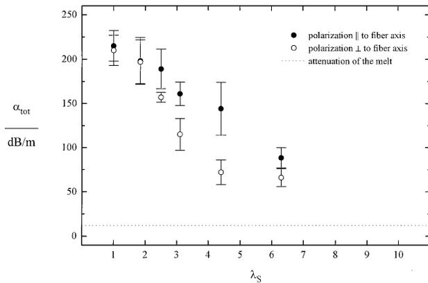
Fig. 3. Attenuation of drawn samples determined by light transmission measurements perpendicular to the fiber axis as a function of draw ratio  $\lambda_S$ . Data are given for polarization parallel and perpendicular to the fiber axis.
