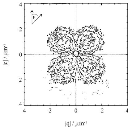
Fig. 5. Depolarized small-angle light-scattering pattern of a melt-crystallized sample as a function of  $q$ .
