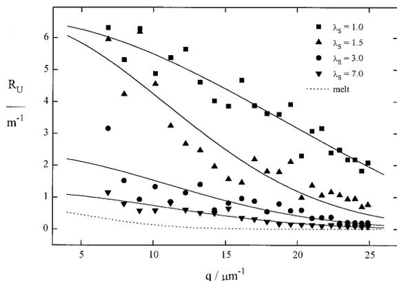
Fig. 7. Rayleigh ratio for unpolarized light of melt-crystallized samples as a function of  $q$ ; the incident light was parallel to the fiber axis. Parameter is the draw ratio  $\lambda_S$ ; the drawn curves are fits of a Debye function to the data points.
