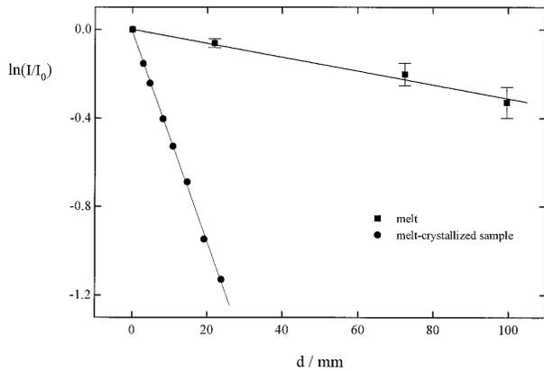
Fig. 2. Light transmission of a molten sample and a melt-crystallized sample as a function of sample thickness.
