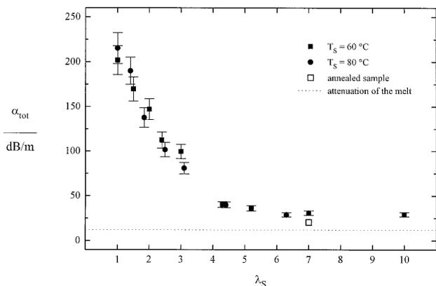
Fig. 4. Attenuation of drawn samples determined by light transmission measurements parallel to the fiber axis as a function of draw ratio  $\lambda_S$  for two different stretching temperatures  $T_S$ .
